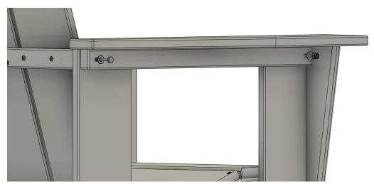
From the inside of the front leg, insert (1) 2-1/4" bolt and secure with a washer and nut. Tigthen the bolt using a 7/16" nut driver bit and handhel drill. Prevent the bolt head from turning by using a #3 Philips screwdriver. Repeat on the other side. Once both arm assemblies are secure, go back and tighten the
