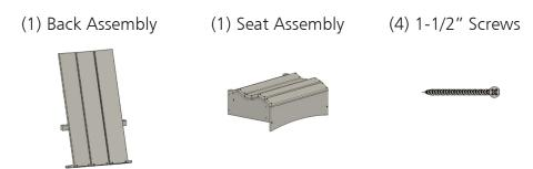
Lay the parts out on a flat, non-abrasive surface to prevent scratching. Align the bottom of the back assembly with the center brace in the seat assembly. Insert (4) 1-1/2" screws into the countersunk holes and tighten using a #2 Philips screwdriver bit and handheld drill.
